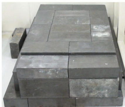
Fig. 19.1 The lead shield employed for detecting the low level of radiation
