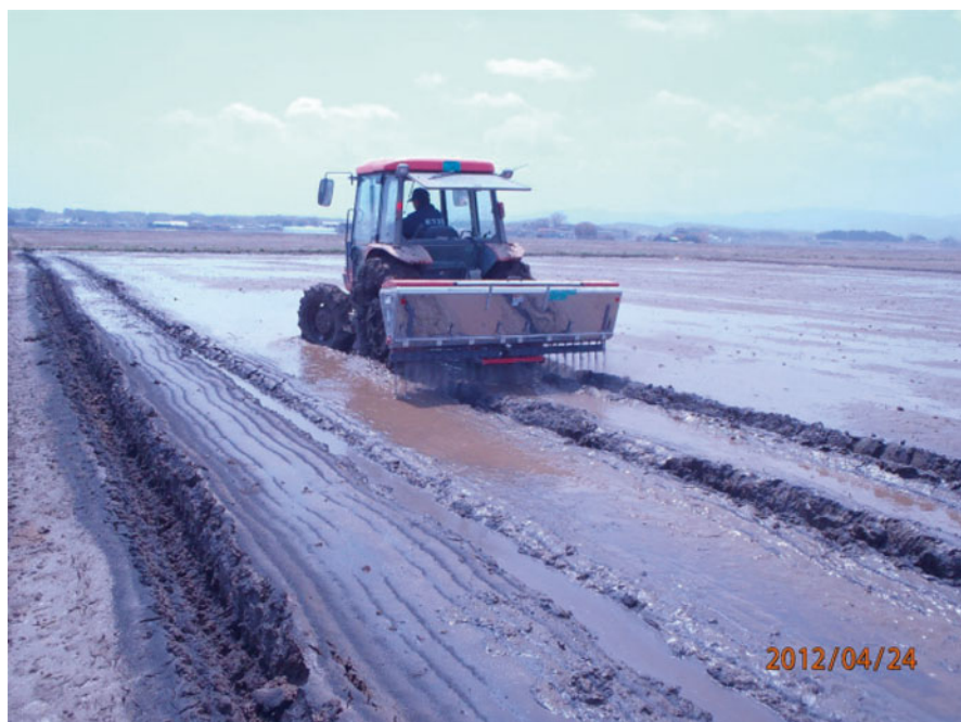
Fig. 4.17 Application of converter slag using lime sower (April 2012)
