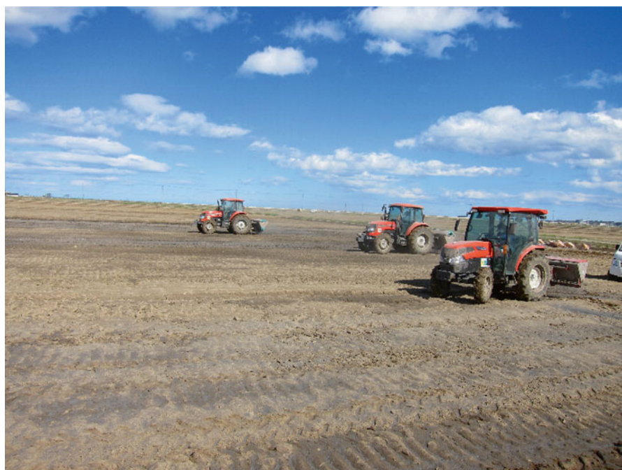
Fig. 4.20 Application of converter slag using lime sower by collaboration of farmers (April 2013)
