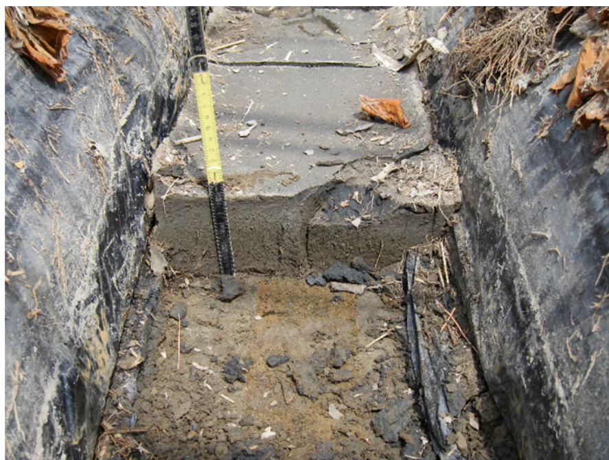
Fig. 4.3 Tsunami sediment deposited on the topsoil of a strawberry greenhouse
