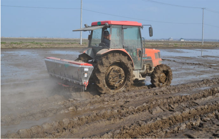
Fig. 17.3 Using a lime sower to spread converter slag
