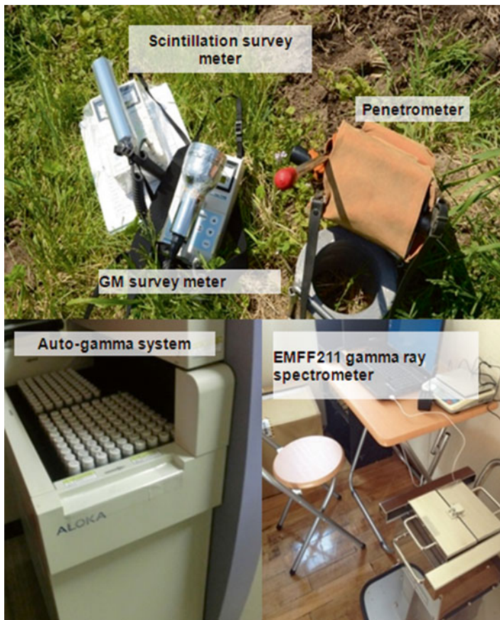
Fig. 10.5 Devices to measure ambient radiation doses and radionuclides
