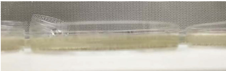
Fig. 3 The agar level should fill the bottom of the petri dish 2/3–3/4 full
