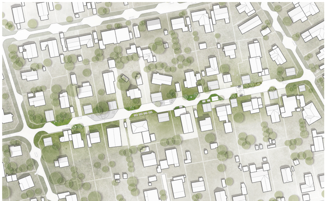
Figure 8. Proposed site plan. Newly inserted buildings and functions operating at different scales disrupt the grid and create a gradient of zones with different levels of privacy.
