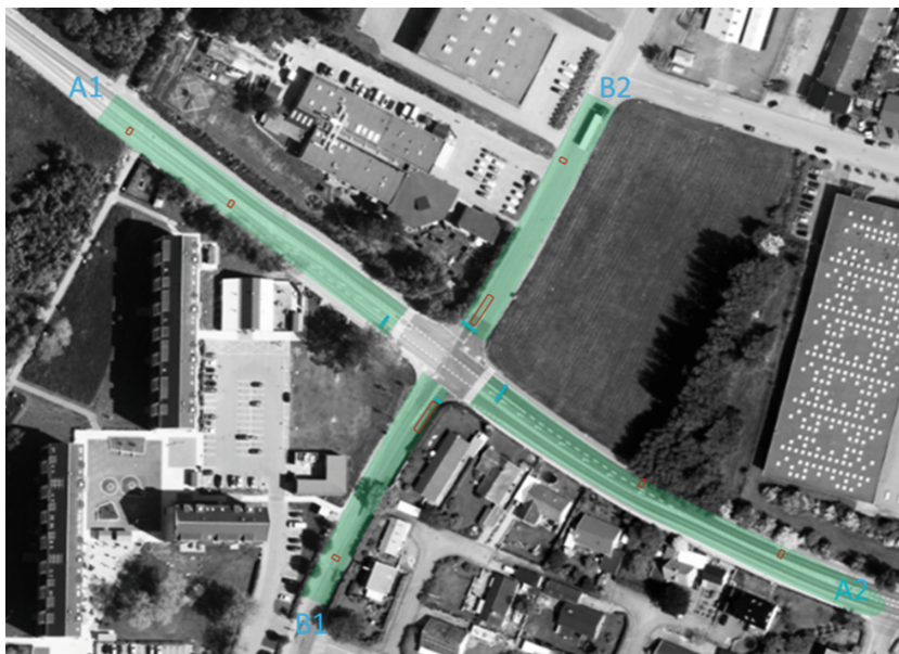
Fig. 11. Intersection between Nylandsvej and Værkstedvej at Køge municipality. Layout of loops and radar area.
