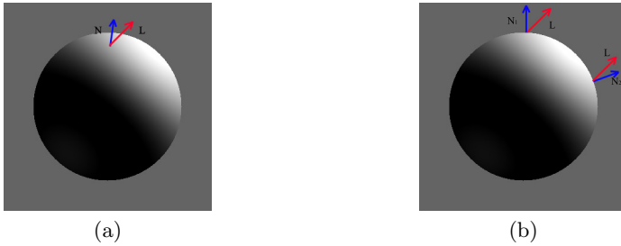
Fig. 1. (a) 3D information extraction from a sphere (b) 2D information extraction along the boundary of a sphere. L denotes the light direction, N denotes the surface normal; N_1 and N_2 are the normal vectors along the occluding contour.
