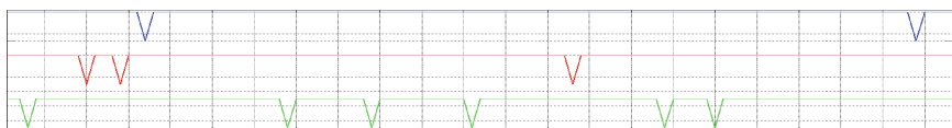
(b) After peak detection (the horizontal axis is the peak/dip number and the vertical axis is “high” for peaks and “low” for dips)
