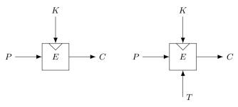
(a) Regular Block Cipher. (b) Tweakable Block Cipher.
