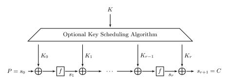
**Fig. 1.** Key-alternating cipher: the function f is applied r times, surrounded by subkey mixing operations
