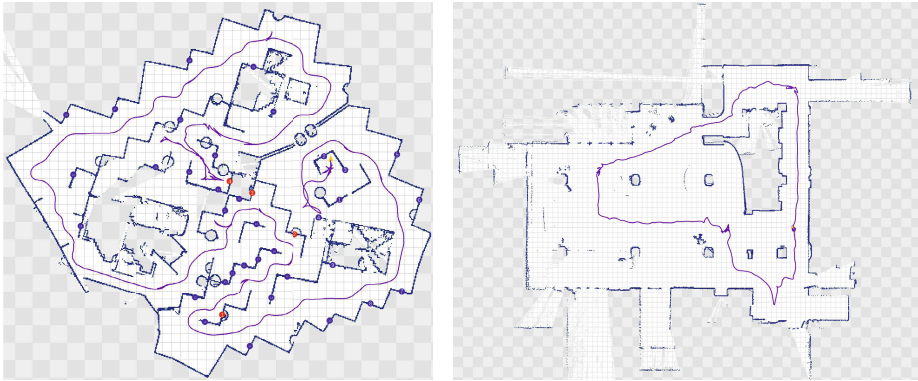
Fig. 4. Maps learned using the provided Hector modules. Left: Map learned using hector_slam and hector_exploration_planner at the RoboCup 2012 final mission with the Hector UGV robot. The robot started at the right middle position and autonomously explored the majority of the arena, finding 3 victims (red markers). The fourth victim was found using tele-operation for the last 4 meters of the travelled path. Blue markers indicate the positions of 35 QR codes that were detected autonomously by the robot. Right: Application of hector_slam to the ccny quadrotor lobby dataset [13].
