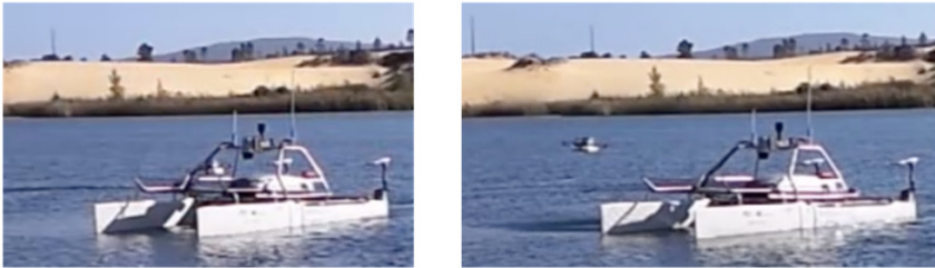
Fig. 6. Field trials: UAV taking off the ASV. Left: moment right after the taking off takes place. Right: A few moments after the take off onset.
