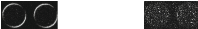
Fig. 9. Error distances (5) to the local gray line for the calibration image of cam 1, before (left) and after (right) correction
