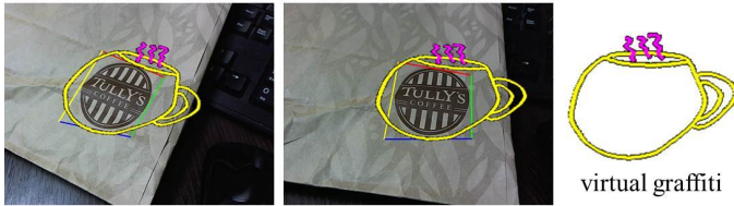
Fig. 13. Marker-less AR application. Virtual graffiti is superposed on live video frames.
