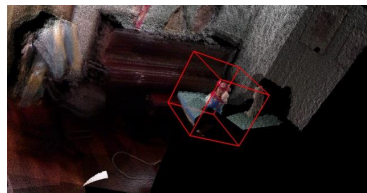
Fig. 6. We moved the camera on a circular trajectory and repeatedly acquired the same loop. TSDF-enabled optimization yields very low drift tracking, while semantic bundle adjustment detects and localizes objects (see the red boxes).
