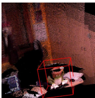
Fig. 6. We moved the camera on a circular trajectory and repeatedly acquired the same loop. TSDF-enabled optimization yields very low drift tracking, while semantic bundle adjustment detects and localizes objects (see the red boxes).
