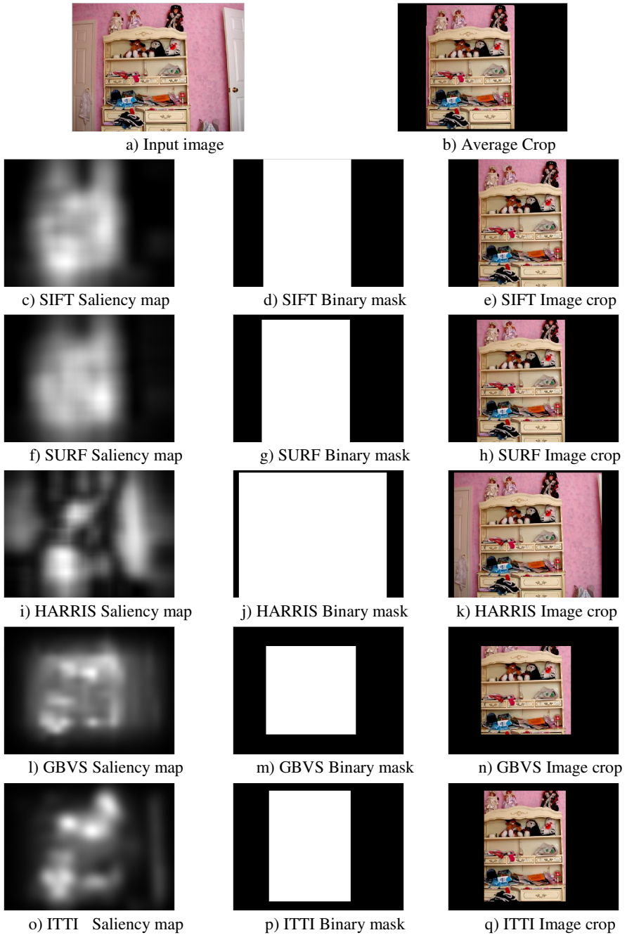
Fig. 7. A visual example of image crops with the different saliency maps. Saliency maps are binarized with threshold = 0.35, which is a good tradeoff for all the methods (see fig. 6)
