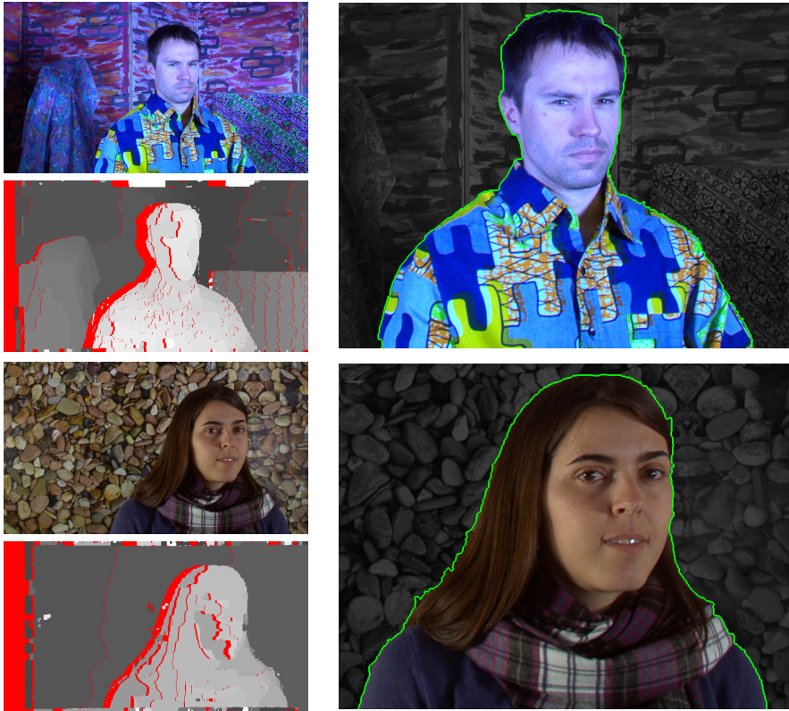
Fig. 4. Segmentation samples from HD stereosequences. The color frames and the disparity maps are shown on the left and the segmented foreground on the right.
