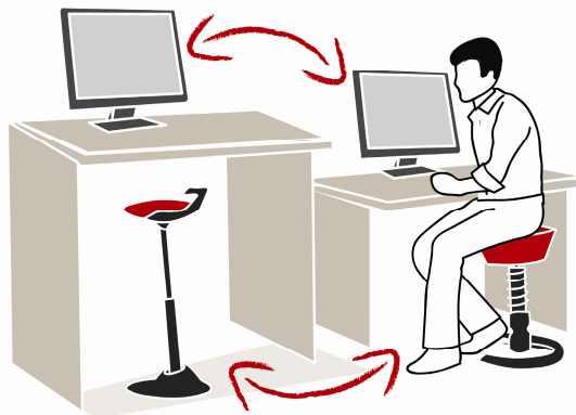
Fig. 1. A sit-and-stand workplace design integrating the concept of working in sitting and standing posture into the daily office workflow
