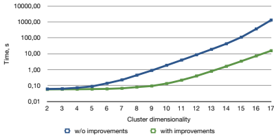
(a) Speed-up due to algorithmic improvements as a function of the cluster dimensionality k .
