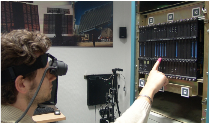
Fig. 5. User wearing HMD and colored fingertip caps
