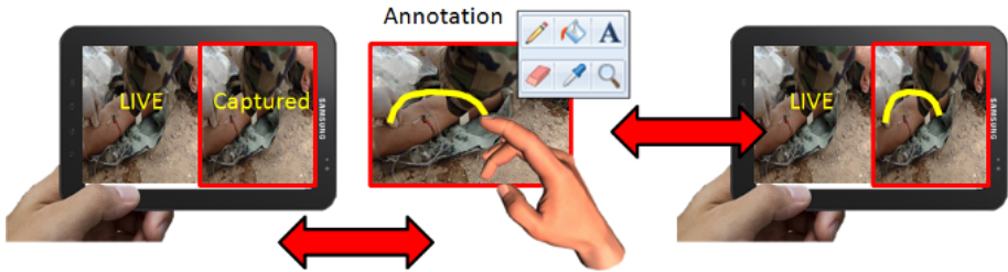
Fig. 1. The Helper captures an image from the Worker's video and annotates it to instruct the user on how to perform a task
