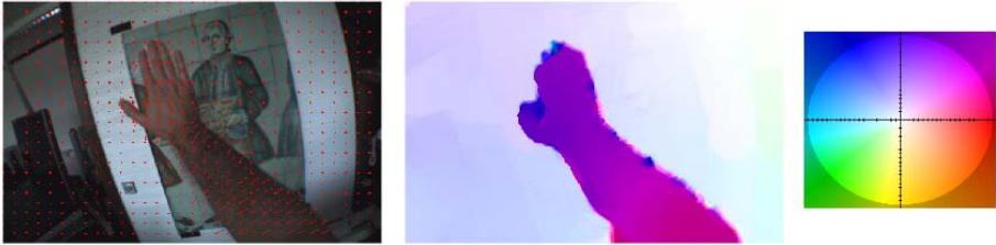
Fig. 2. Left: Hand with overlaid motion vectors. Middle: Color-coded dense flow field. Right: Color wheel for color-coding flow vectors [3].
