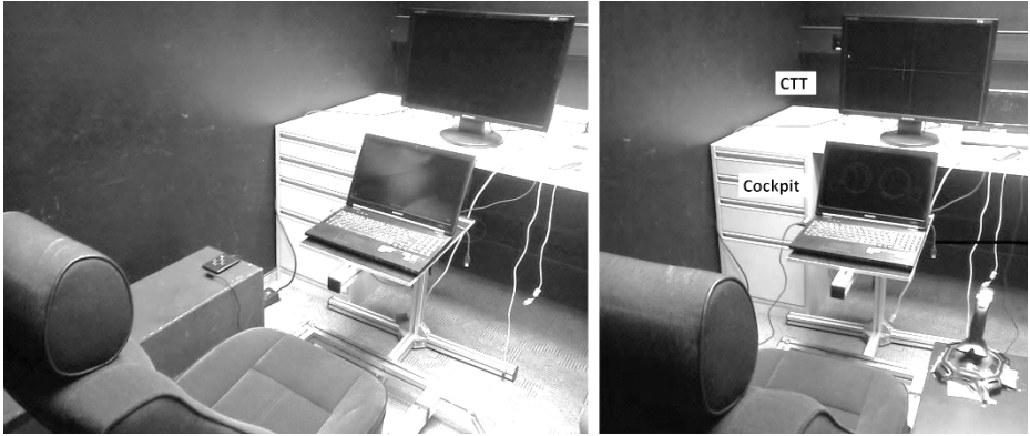
Fig. 3. Experimental setting of experiment 1. Participants sat in a car seat and performed two tasks simultaneously. All distances were recreated based on a real car.
