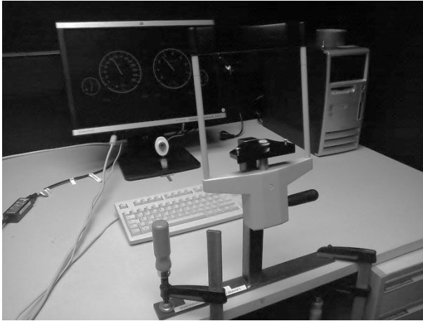
Fig. 4. Set-up of Experiment 2. Participants sat on a chair with the head resting on a chin rest while pictures with cockpit displays showing different speeds were presented on the screen.
