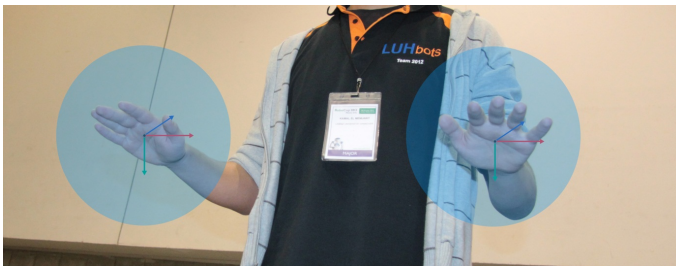
Fig. 6. Hand gesture control of the robot - two coordinate frames are placed inside the user's hand
