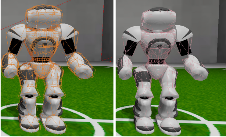
Fig. 4. The left picture shows the PhysX collision model, the right picture the Unreal Engine collision model
