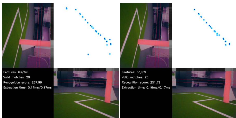
Fig. 2. Left: Matching features in two similar images based on nearest neighbour (NN) matching. Right: Matching features in the same two images after using RANSAC to discard matches that don't agree on a consistent pose (NN with RANSAC). As in Figure 1, each image displays the horizon band in red and the extracted grey-scale horizon pixels at the top of the image. Matching features are plotted in the top-right panel against their horizon location in each image. The text panel illustrates the number of features detected in each image, the number of matches, the recognition score and the time taken to extract the features on a 2.4GHz laptop.
