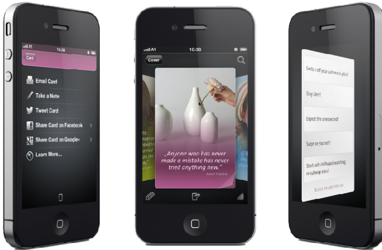
Fig. 3. Early 2012 prototype of CardSkid UI. The device in the center depicts a deck of cards zoomed out into an overview, providing additional visual cues for navigation. On the left screen, a card has been pushed up to reveal a list of contextual actions. On the right screen, a card is being flipped over to show additional content on its back.
