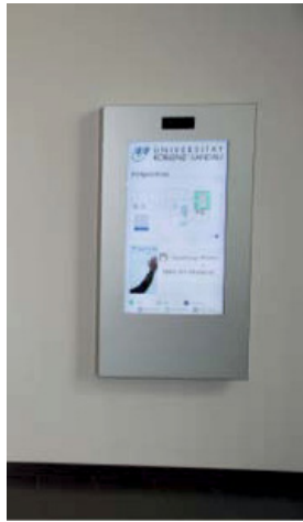
Fig. 1. Wall-mounted gesture control floor navigation system
