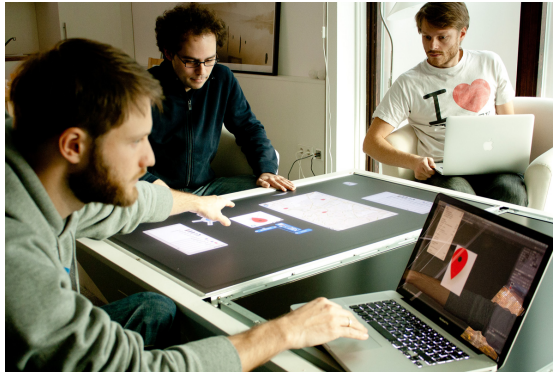
Fig. 1. Three authors modifying a prototype in the EMIL authoring application on a tabletop system. In the foreground, a UI designer modifies the image of a map marker in Photoshop on his computer. As soon as the UI designer saves the Photoshop file on his laptop to the cloud storage, the changes become available in the prototype and all components that contain the marker resource from Photoshop can be updated.
