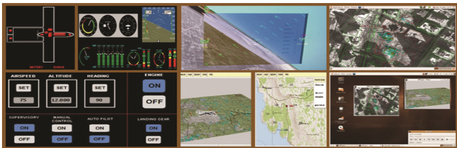
Fig. 3. Proposed GUI for Sky-eye two-wing UAV
