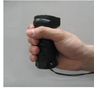
Fig. 2. Vibration alert interface. Length is 10cm, diameter is 3.5cm. A compact DC motor is mounted in the device.
