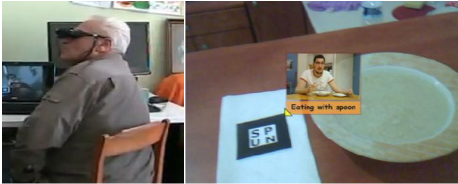
Fig. 3. Using AR glasses (left), SymbioSpace provides to the user additional information for simple tasks, e.g., eating with spoon (right)
