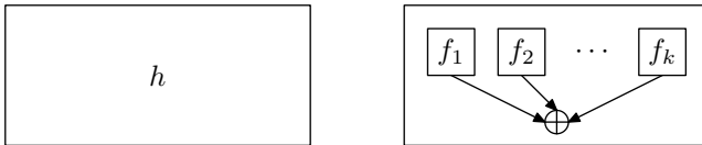
Fig. 1. Our attack distinguish between a function and the xor of k permutations
