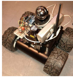
Fig. 1. RobAIR - platform and sensors (geiger, toxic gaz)
