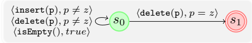
Fig. 2. An observer for checking that no data value can be deleted if it has not been first inserted. The variable z is an observer variable.
