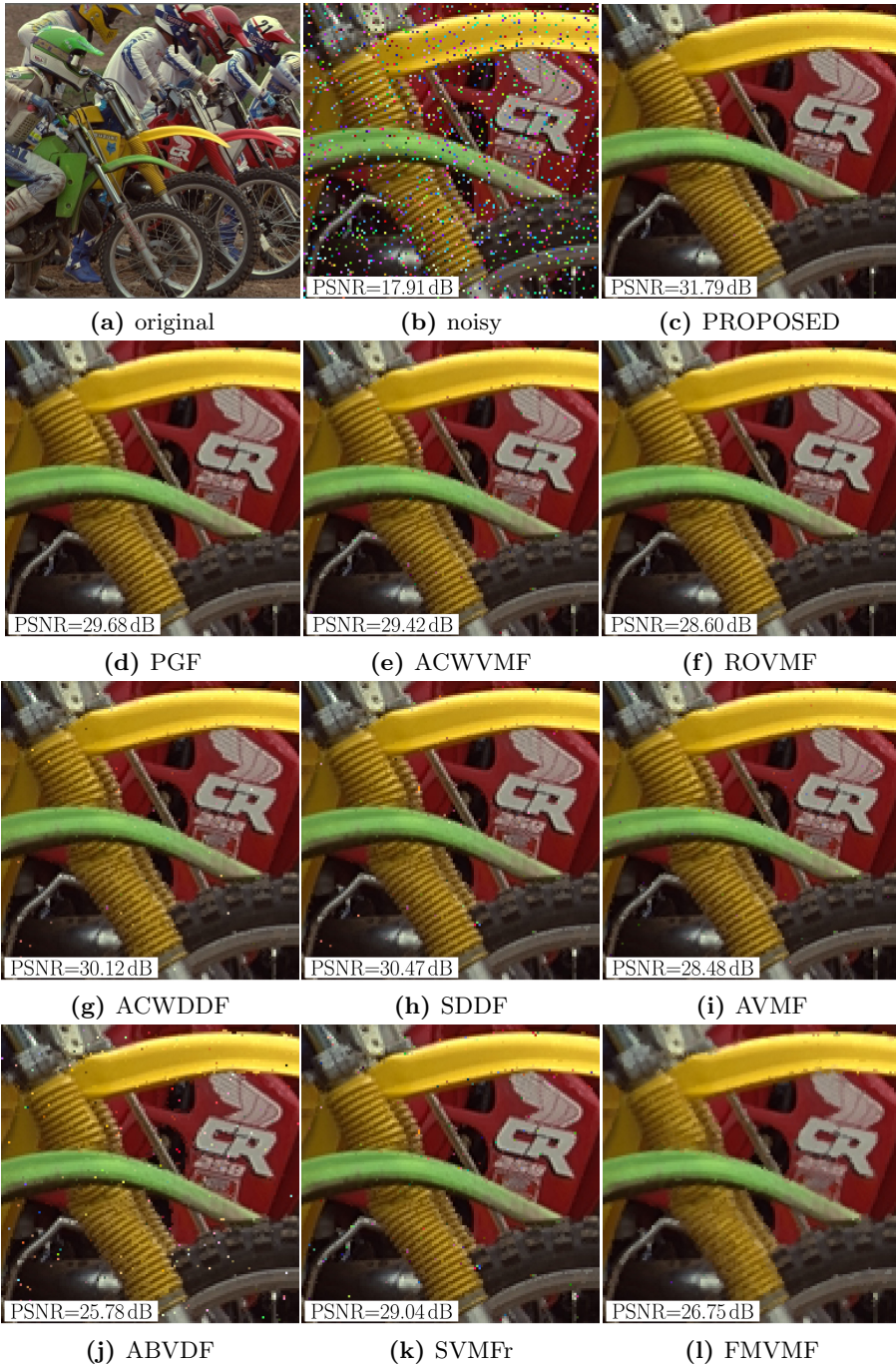
Fig. 8. Comparison of the efficiency of the proposed switching filter as compared with the standard methods, using the color MOTORCROSS image corrupted by impulsive noise with intensity p = 0.1
