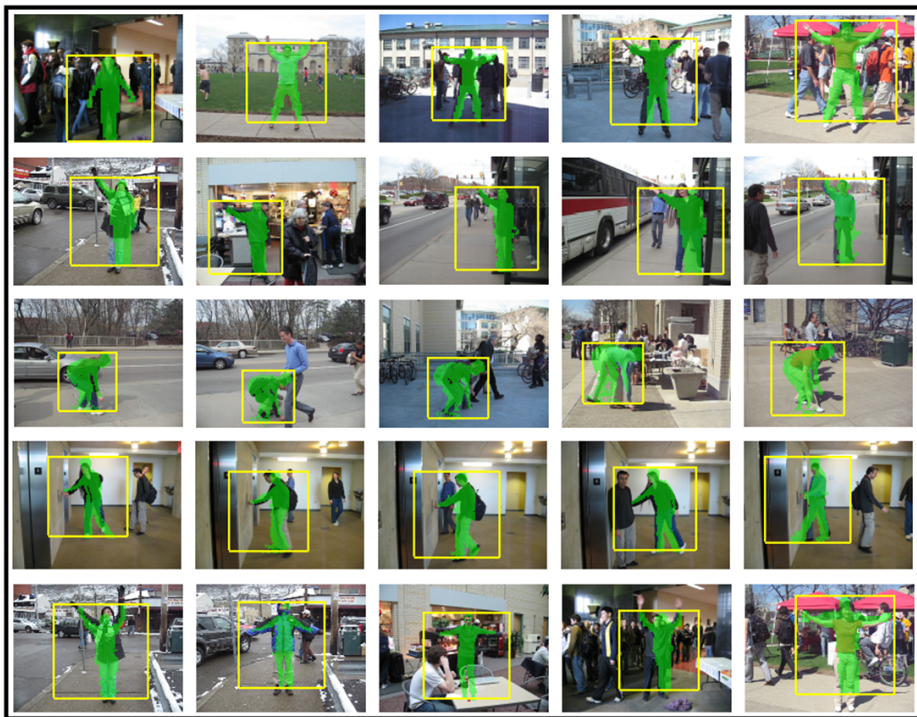
Fig. 7. Examples of action localization and recognition results on the CMU dataset. Note that our approach effectively handled interruption of moving people and vehicles in the scene. The 1 st row: jumping-jacks; The 2 nd row: one-handed-wave; The 3 rd row: pick-up; The 4 th row: push-button; The 5 th row: two-handed-wave. The green regions are the segmentation masks.
