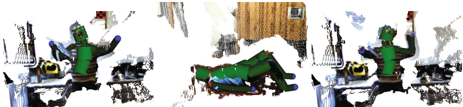
Fig. 1. The type of articulated tracking for which we achieve a speed up factor of up to 600 when using a GPU optimization. The images show stereo points with a superimposed illustration of the skin model.
