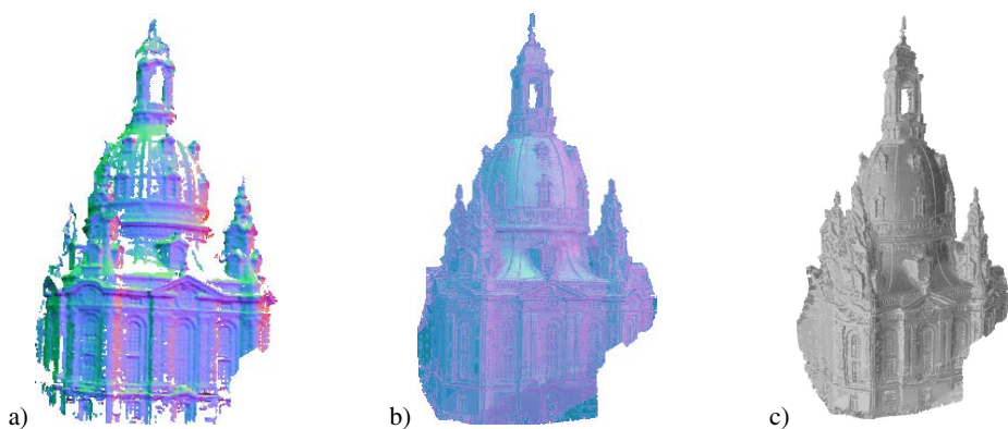
Fig. 10. Cathedral model. a) Normal map of partially reconstructed geometry using multi-view stereo serving as scene-intrinsic reference geometry (SIRG), b) reconstructed normal map, c) final model rendered from novel viewpoint.
