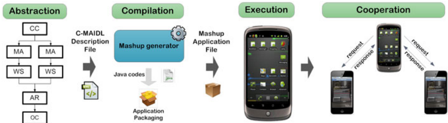
Fig. 2. Mashup Construction Process
