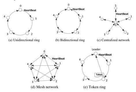
Fig. 1. Classical node failure detection models
