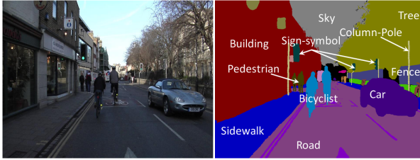
Fig. 1. Semantic scene segmentation aims at assigning every pixel in an image by one of the predefined semantic labels available (i.e., pedestrian, car, building, road, sidewalk, tree, sky). Image taken from [3].
