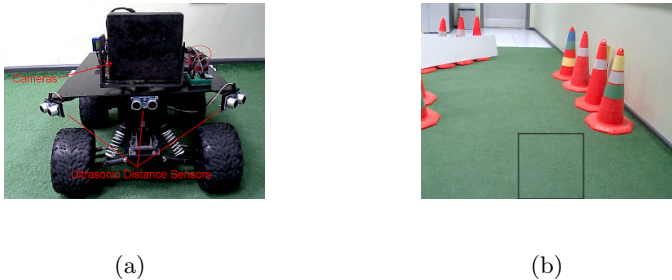
Fig. 1. (a) Model car equipped with camera and sensors (b) Obstacle free region
