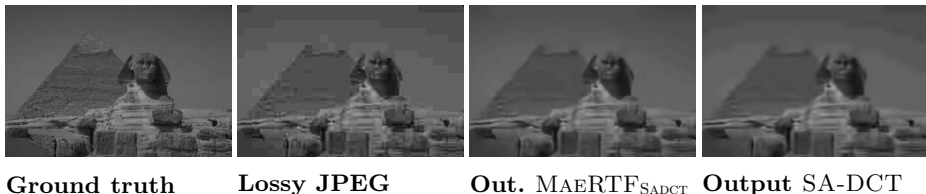
Fig. 8. Improvement in JPEG deblocking (quality 10): SA-DCT fails to remove the blocking artefacts in the sky while our MAERTF SADCT -system succeeds
