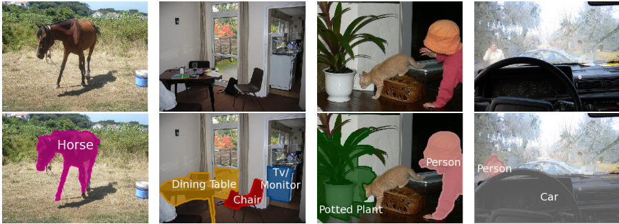
Fig. 1. Examples of our semantic segmentations including failures. There are typical recognition problems: false positive detections such as the tv/monitor in the kitchen scene, and false negatives like the undetected cat. In some cases objects are correctly recognized but not very accurately segmented, as visible in the potted plant example.
