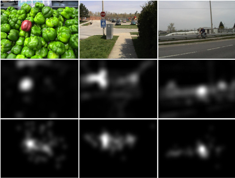
Fig. 1. Saliency from the color co-occurrence histogram (CCH): For the sample images in the first row, the second and the third rows show the corresponding CCH based saliency maps and fixation maps, respectively
