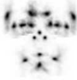
Fig. 2. Superposition of vote accumulation images for 17 point face model. Note that there is a separate image for each point.
