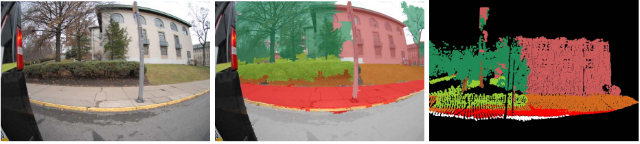
Fig. 1. Multimodal scene analysis. The reference scene (left) is observed with a camera and laser scanner and simultaneously classified in the image (middle) and 3-D point cloud (right). Color code: dark-red=sidewalk, white=road, light-green=shrub, dark-green=tree-top, brown=tree-trunk, light-red=building.
