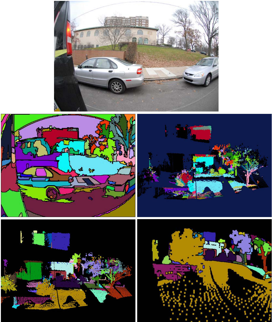
Fig. 3. The effects of constraining the representation into a single domain. Top (a): Reference scene. Middle (b): 2-D driven approach. The image is segmented (left) and then back-projected into the 3-D point cloud (right) using occlusion reasoning. The 3-D region colors correspond to the 2-D segmentation, except the 3-D points colored black which are occluded with respect to the camera's viewpoint and are not associated with any 2-D region. Bottom (c): 3-D driven approach. The original 3-D point cloud is segmented (left) and then projected into the image plane (right) using occlusion reasoning. Note that not every pixel is associated with a 3-D region and that the resulting 2-D regions are not connected due to occlusions, and sampling rates.
