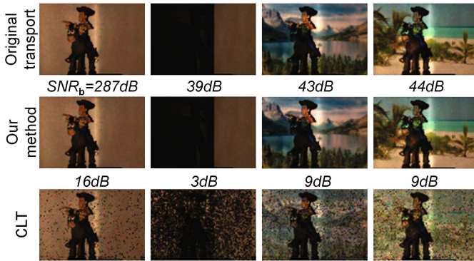
Fig. 6. We compare our method with CLT [9] under four relighting examples. Both methods acquire 6800 \times 6800 transport matrix using 423 patterns. Our method significantly outperforms CLT since CLT is not designed for spatially varying illumination.
