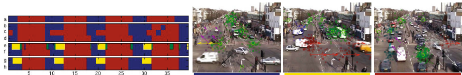
Fig. 7. Junction dataset. (a) Ground truth annotation [25] and temporal segmentation results obtained with (b,c) standard and hierarchical pLSA [25], (d) EMP [5], (e,f) DDP-HMM [3] and (g,h) our method. (Left) extracted high-level activities \omega_m = 0.9 .
